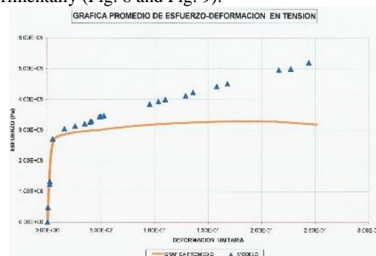
Figure 8. Comparative graph of the real values obtained in the experimentation, against the values calculated by the mathematical model in the tensile deformation process. The graph shows the average experimental stress-strain curve.
