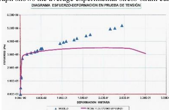
Figure 9. Comparative graph of the real values obtained in the experimentation, against the values calculated by the mathematical model in the tensile deformation process. The graph shows the experimental stress-strain curve for specimen 17, which records the maximum stress
