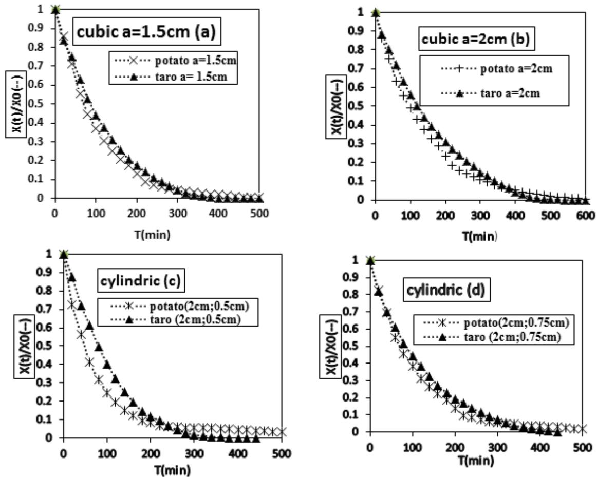
Fig 3. Influence of the nature of products on the drying of cubic samples (a), (b) and cylindrical samples (c), (d)
