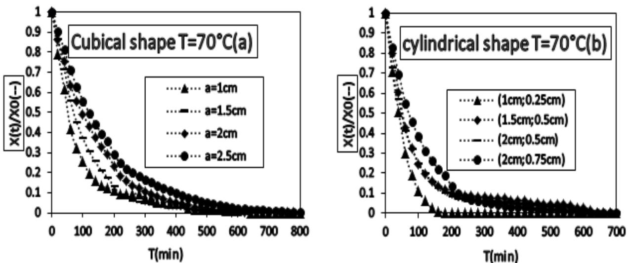
Fig 1. Effect of size on drying kinetics of potato samples: cubical (a) and cylindrical (b)
