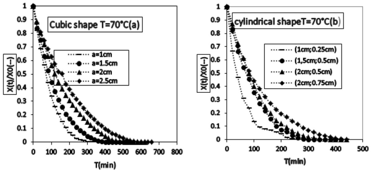
Fig 2. Effect of size on drying kinetics of taro samples: cubic (a) and cylindrical (b)
