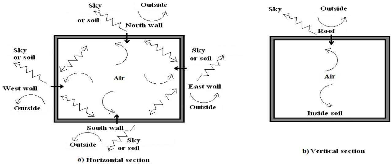
Figure 2. Diagrams of the different heat exchanges in the habitat [9]
