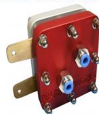
PROTO TYPE ONE CELL PEM FUEL CELL STACK WITH GOLD PLATED ALUMINIUM
