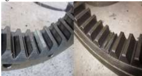
(i) Tooth worn face (ii) Broken gear Fig3. Two common faults of gears
