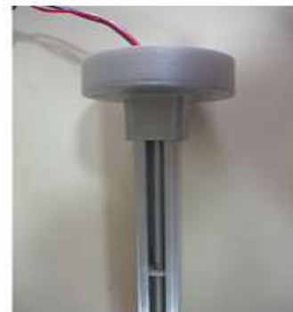
Figure 2. Physical View of Capacitive Fuel Level Sensor
