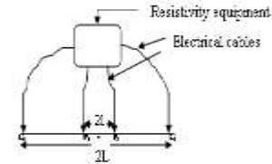
**Figure 4 Resistivity Sounding Set-Up**
