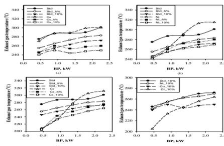
**Figure 4 Variation of exhaust gas temperature with brake power for different EGR flow rate and coatings**
