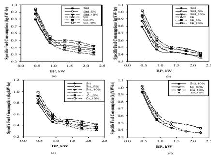
**Figure 3 Variation of specific fuel consumption with brake power for different EGR flow rate and coatings**
