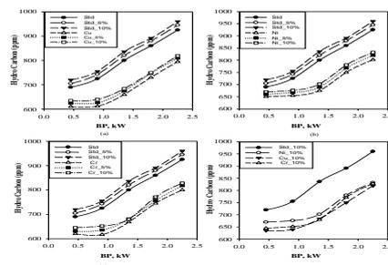
**Figure 7 Variation of Hydro Carbon (ppm) with brake power for different EGR flow rate and coatings**
