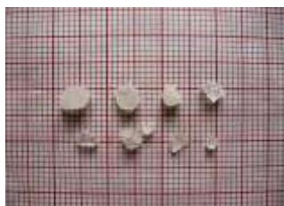
Fig. 2 Photograph of the KNB crystal grown in water
