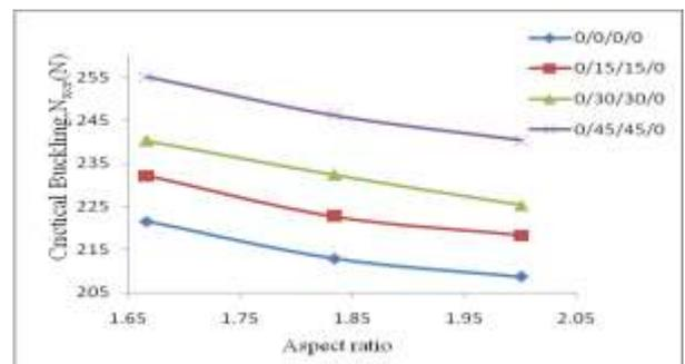
**Fig. 11. Effect of L/W and  $\theta$  on buckling strength of thin composite plate having anti-symmetric layup with CCCC boundary conditions.**
