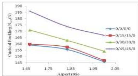
**Fig. 8. Effect of L/W and  $\theta$  on buckling strength of thin composite plate having symmetric layup with CCSS boundary conditions.**
