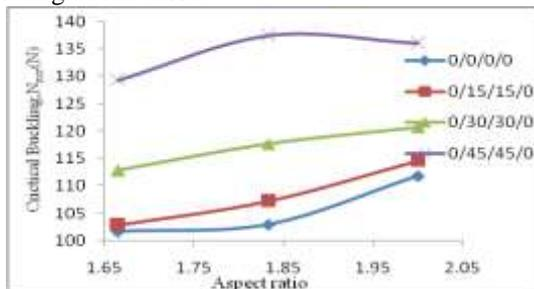
Fig. 6. Effect of L/W and  $\theta$  on buckling strength of thin composite plate having symmetric layup with CSSS boundary conditions.
