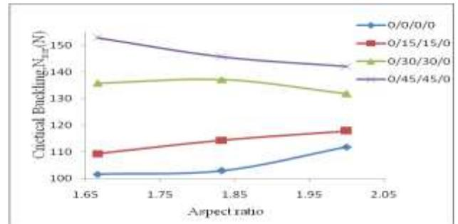
Fig. 7. Effect of L/W and  $\theta$  on buckling strength of thin composite plate having anti-symmetric layup with CSSS boundary conditions.
