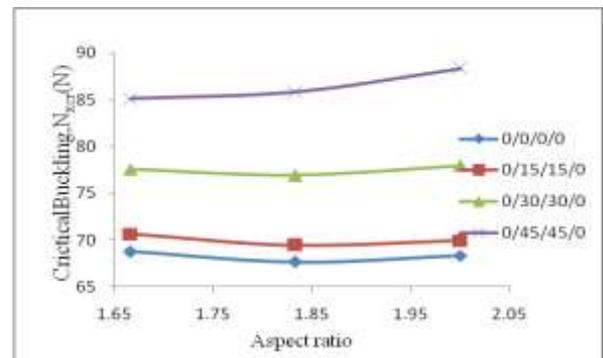
**Fig.4. Effect of L/W and θ on buckling strength of thin composite plate having symmetric layup with SSSS boundary conditions.**
