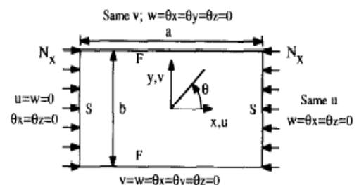
Fig. 1. Loading and boundary condition applied for validation of FE model
