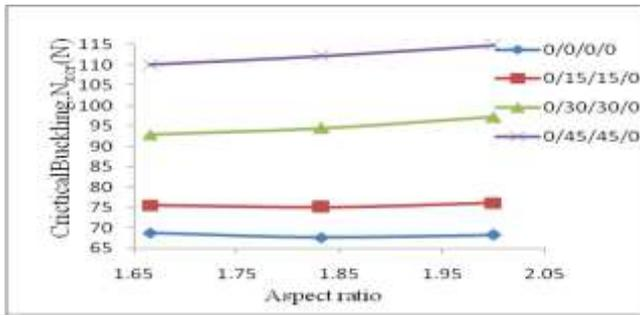
Fig. 5. Effect of L/W and  $\theta$  on buckling strength of thin composite plate having anti-symmetric layup with SSSS boundary conditions.
