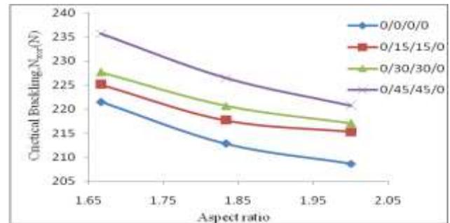
**Fig. 10. Effect of L/W and  $\theta$  on buckling strength of thin composite plate having symmetric layup with CCCC boundary conditions**
