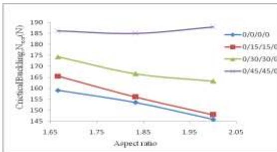
**Fig. 9. Effect of L/W and  $\theta$  on buckling strength of thin composite plate having anti-symmetric layup with CCSS boundary conditions.**
