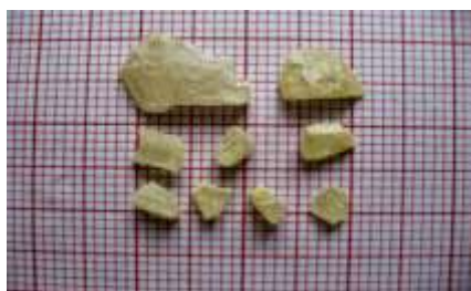
Fig 2. Photograph of the 2MN crystal grown in methanol
