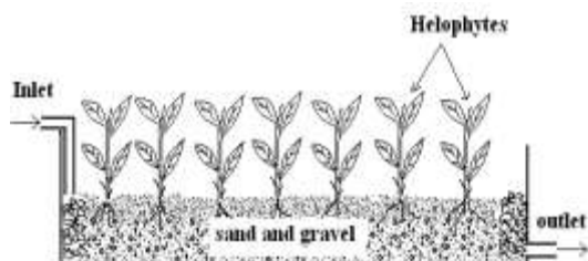
Figure 2: Subsurface flow constructed wetland
