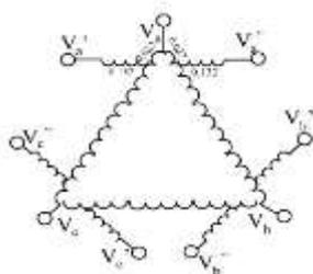
Fig.3. Proposed autotransformer winding connection diagram.
