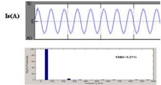
Fig.9. AC mains current waveform along with its harmonic spectrum at full load with 18-pulse ac-dc converter on ac side
