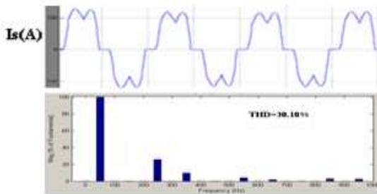
Fig. 7. AC mains current waveform along with its harmonic spectrum at full load in a six-pulse diode bridge rectifier-fed VCIMD.
