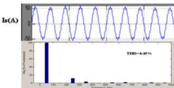
Fig.8. AC mains current waveform along with its harmonic spectrum at full load with 12-pulse ac-dc converter on ac side
