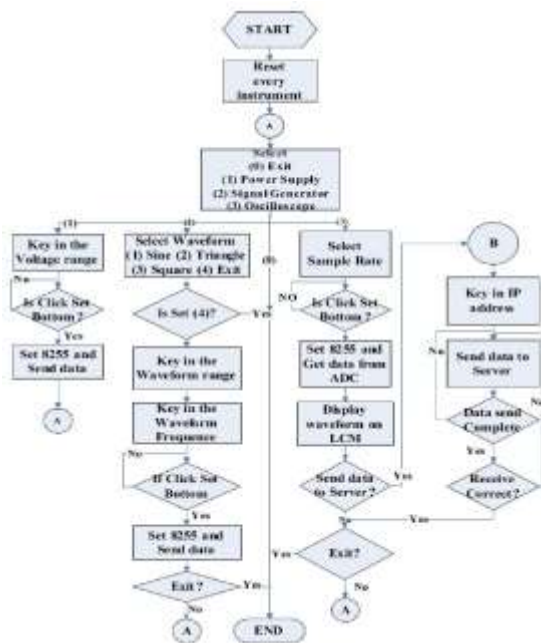
Fig 9. The flowchart of the embedded remote electronic measurement system
