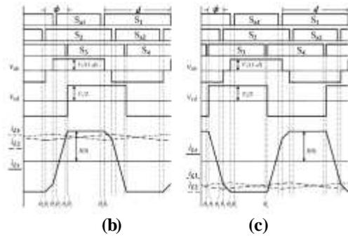
Fig 1.(a) power circuit of conventional bidirectional dc-dc converter.(b) Key theoretical waveforms in (b) Boost mode and (c) Buck mode.
