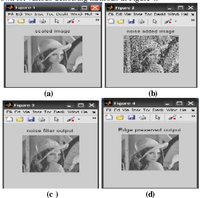
Fig 4: Results of SEPD in MATLAB, (a) Noise-free image; (b)Noisy image; (c)Noise Filter output; (d) Edge Preserved output
