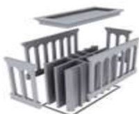
Fig. 6. 3D model of a Wind catcher with different canals [Roaf, 1989]
