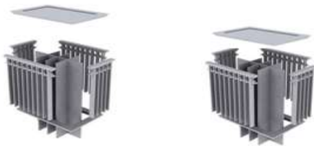
Fig. 4. 3D model of a Wind catcher with equal canals . [Roaf, 1989]
