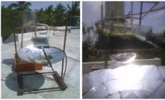
Fig. 3 Pictorial view of rose water distillation unit and Rose water container gets the heat flux from concentrator
