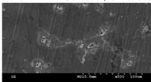
Figure 5 SEM images obtained for the mild steel surfaces immersed for 2 h in 1M Citric acid with 36.85mM inhibitor solution
