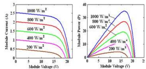
Fig.2 Simulated V-I and V-P Characteristics of SPV module for Various Insolation at Constant Temperature  $T=250C$
