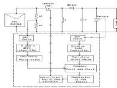
Fig. 10 Hardware Schematic of the Proposed Controller
