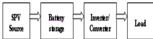
Fig.1 Structure of Standalone System
