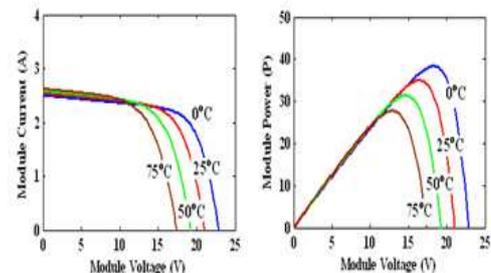
Fig. 3 Simulated V-I and V-P Characteristics of SPV module for Various Temperature at Constant Insolation  $G = 1000W/m^2$
