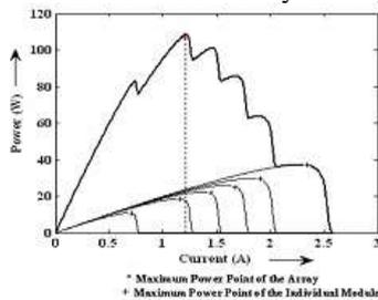
Fig. 5 V-P Characteristic for Series SPV Configuration Converter Selection
