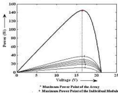
Fig. 4 V-P Characteristic for Parallel SPV Configuration
