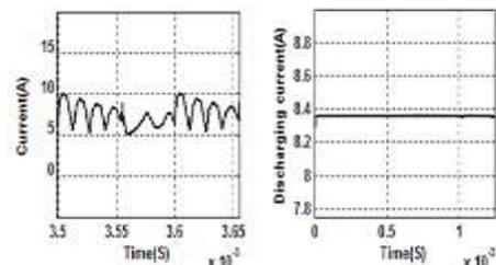
Fig. 9 Charging and discharging currents of the battery
