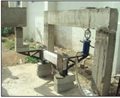
Fig. 1 Typical setup for Shear and Torsion Test
