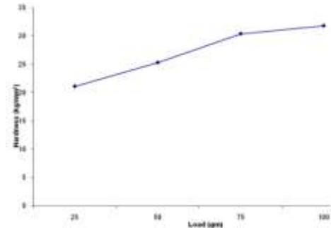
Fig.7 Plot of Load Vs Hardness of MPHb crystal SHG efficiency measurement
