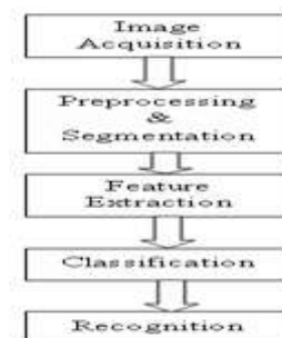
Fig. 3: A general diagram for handwritten digit recognition
