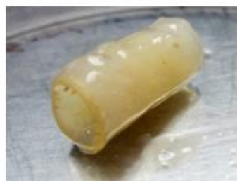
Figure -1 shows the picture of chitosan dip coated silicone catheter using PDLA as crosslinking agent
