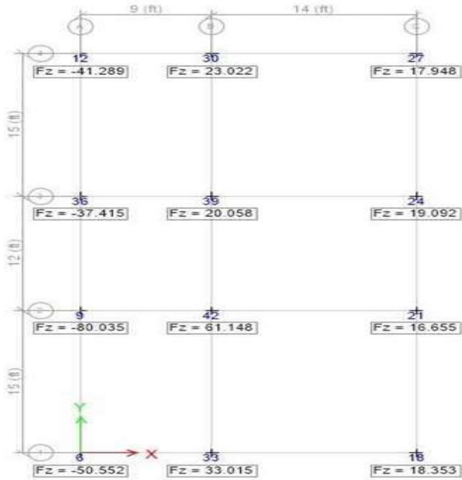
Fig 18. Restraint reaction (Base) X-axis zone-1 ZONE-1 (CHAPAINAWABGANJ) Comparison For Restraint Reaction, Eq x
