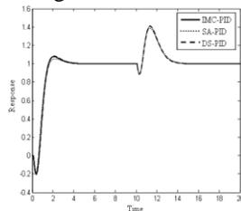
**Fig 1. Comparison of servo problem and regulatory response of constant volume CSTR carrying out Van de Vusse reaction for linear model**
