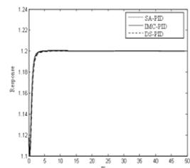
**Fig 2. Comparison of servo problem of constant volume CSTR carrying out Van de Vusse reaction for change in product concentration  $C_B$  from 1.117 to 1.2 gmole/l for non-linear model**
