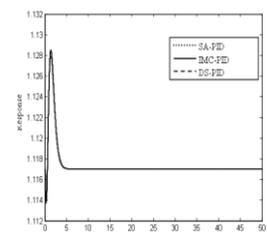
**Fig 3. Comparison of regulatory problem of constant volume CSTR carrying out Van de Vusse reaction for change in ratio of feed flow rate to volume of reactor ( $F/V=0.5714$  to  $0.6 \text{ min}^{-1}$ ) for non-linear model in case study-5.**
