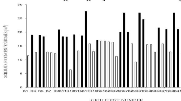
Figure 5. A bar chart of average soil radon gas concentrations against grid point locations at Kwabenya
