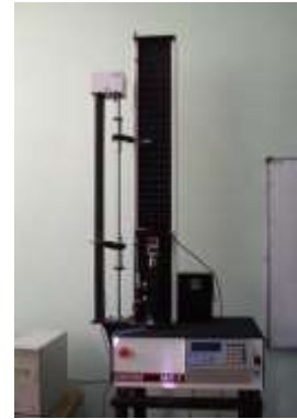
Fig. 1. Universal Testing Machine (Santam, SMT-5) used to determine modulus of elasticity
