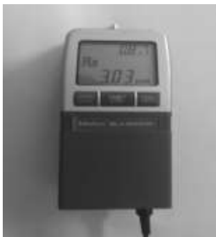
(c). Talysurf surface meter
