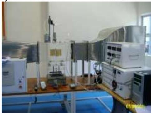
Figure 3 wind turbine model test in wind tunnel
