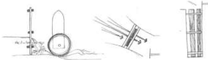
Figure 7. View of the watermill sluice gate (right), the plan sluice gate of watermill (center), profile of the watermill sluice gate (left)
