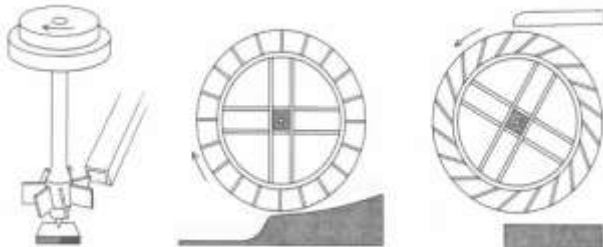
Figure 2. Watermill designs in order to increase complexity and efficiency, Norse watermill (left), under-shot wheeled watermill (center), and over-shot wheeled watermill (right)
