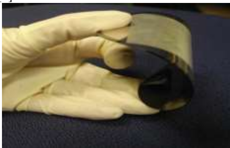
Figure6a. Prototype FSS structure on flexible substrate. [1]
