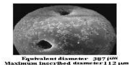
Figure 2. Nano CT – scan showing internal pore structure of a porous pellet (A5)
