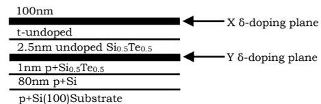
Fig.1 Schematic of the basic Si-based RITD structures with thickness varied from (2.5-25 nm)
