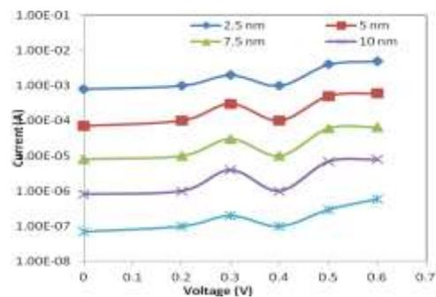
Fig.4. Current and Voltage characteristics of RITDs
