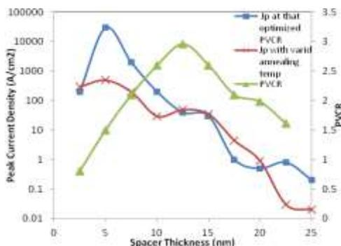
Fig.3. The effect of spacer thickness on PCDs and PVC.
