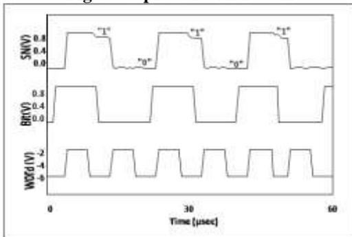
Fig.7. Oscilloscope image of the measured waveforms from the word line, Bit line, and the resulting SN, showing the 1T TSRAM WRITE functionality
