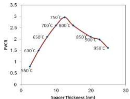
Fig.2 The relation between PVCR and the spacer thickness
