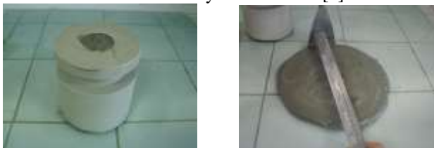
Figure 3.1 Determining consistency of micro concrete
