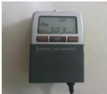
Figure 1 (c). Talysurf surface meter
