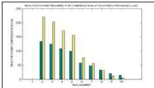
Fig.1: 10-bus radial distribution system which requires the optimal reactive rating of the capacitor to be placed at each bus with the lower load (base) and the upper load (150% of base load).
