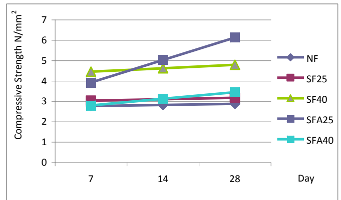
Figure 1: Compressive strength of steel fibre concrete.
