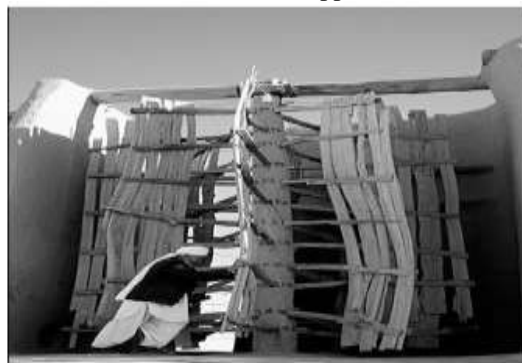
Figure 7. The wind, passing the wind catcher gate, reached the corners of eight-folded ports and moved the wheel and sails.
