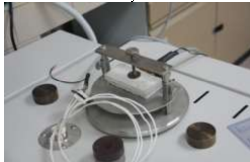
Figure 1: Set-up on Hot disk thermal constant analyzer for thermal test
