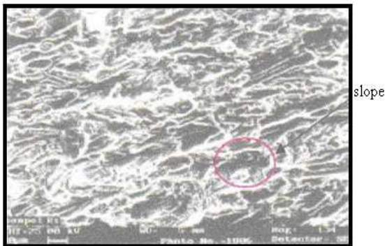
Figure 4.2c: Photomicrography fracture surface for catastrophic failure
