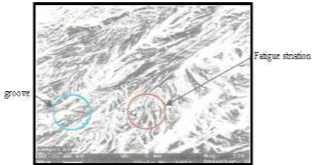
Figure 4.2b: Photomicrography fracture surfaces for crack propagation
