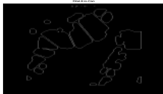
Fig 3.13, shows the thin edges of the farmland's boundaries after the edge and morphological operations
