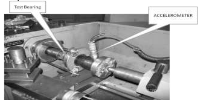
Figure.1 Experimental Setup with Test Bearing and Accelerometer
