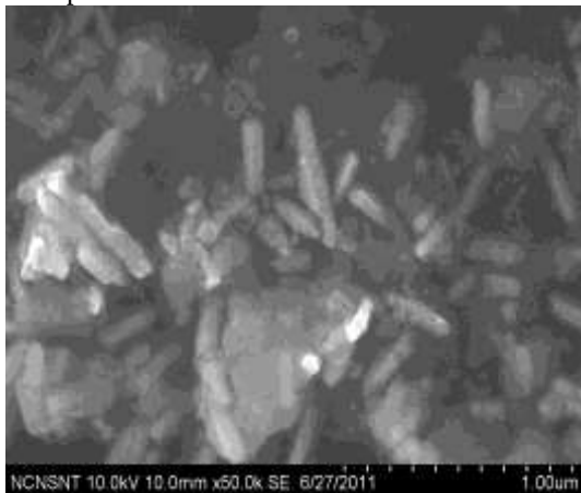
Figure 4 : FE-SEM images of the as-synthesized ZnO/Al 2 O 3 nanoparticles
