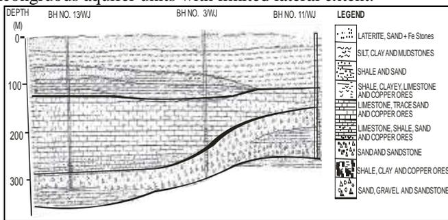
**Figure 4. Lithologic Cross Section deduced from borehole**
