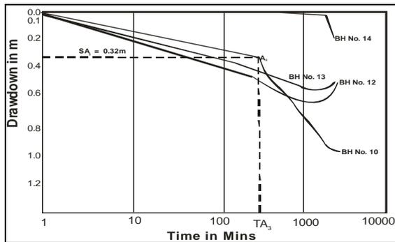
**Figure 9. Simultaneous Constant Rate Pumping Test Result Plots of Bhs. 10, 12, 13 and 14 (Observation Wells)**
