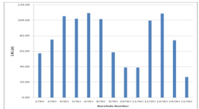
**Figure 6. Static Water Level Record of Boreholes in the Wuro Juli Well Field**
