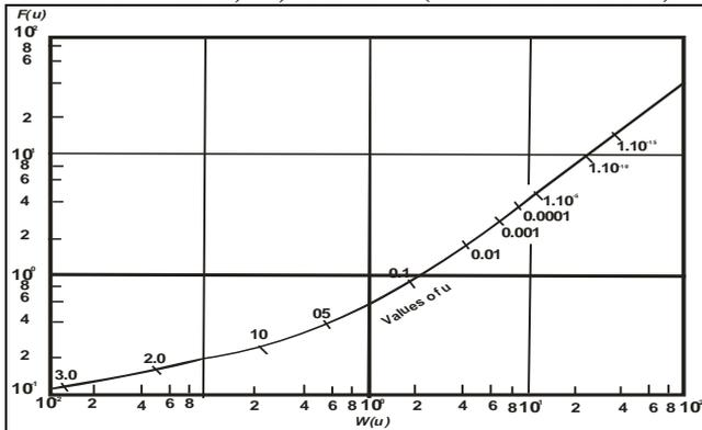
**Figure 10. Chow's Nomogram used for Pumping Test Analysis**
