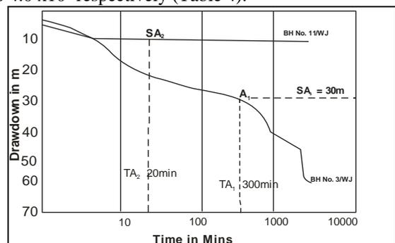
**Figure 8. Simultaneous Constant Rate Pumping Test Result Plots of Bh. 3 and Bh. 11 (Pumping Wells)**
