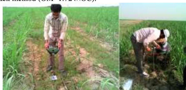
Figure 3. Applying the penetrometer instrument in study fields
