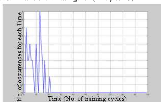
Fig. 11: Illustrate error correction performance with time factor when #neurons = 14, Learning rate = 0.1 and gain factor = 0.5
