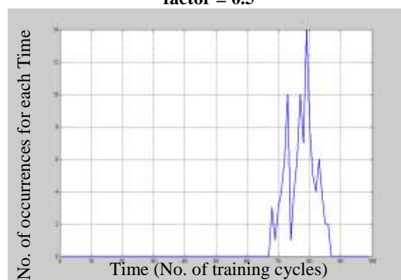
Fig. 14: Illustrate error correction performance with time factor when #neurons = 5, Learning rate = 0.1 and gain factor = 0.5
