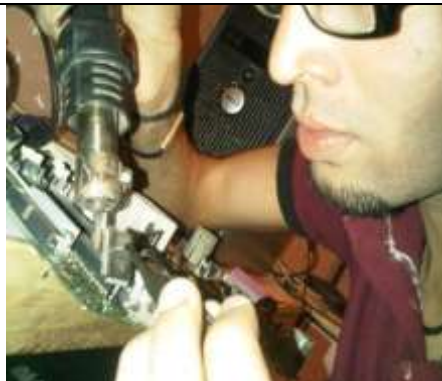
Fig No.12: Remove SMSC Chip
