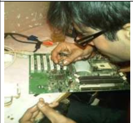
Fig No.13: Remove BIOS Chip
