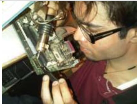
Fig No.9: Heat on SMSC Chip
