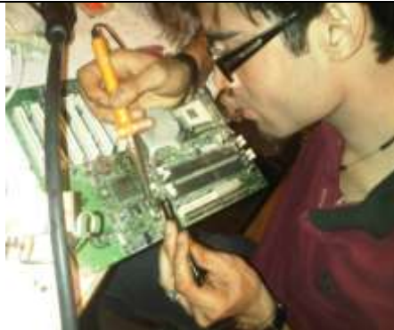
Fig No.3: Soldering the Capacitor
