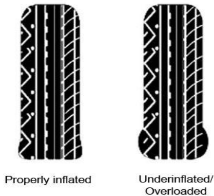
Fig 1. A properly inflated tire and an under inflated or overloaded tire.
