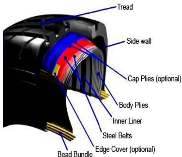
Fig 3. Cross Sectional View of Tire.
