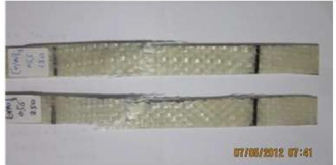
**Figure (2-4) Examples of tensile specimens after failures**
